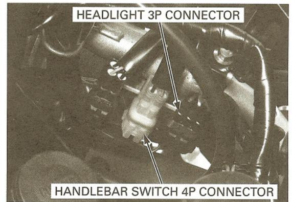
Check for continuity between the switch side connector terminals in each switch position. Continuity should exist between the color coded wires as shown below:
