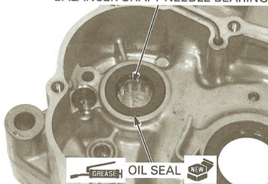
BALANCER SHAFT NEEDLE BEARING
