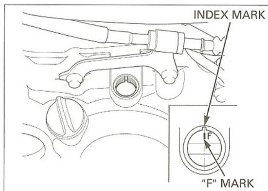
Coat a new O-ring with oil and install it onto the timing hole cap.
