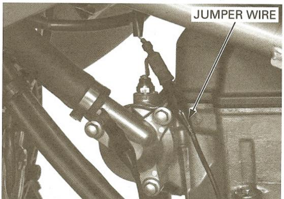
If the wire is OK, disconnect the indicator 2P red connector.
