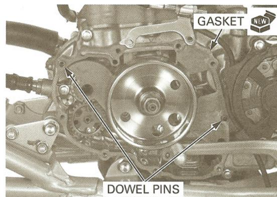
Install the left crankcase cover and cable holder, and tighten the nine bolts in a crisscross pattern in 2 or 3 steps.
