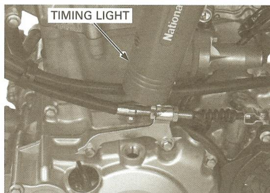
The ignition timing is correct if the "F" mark on the flywheel aligns with the index mark on the left crankcase cover.
