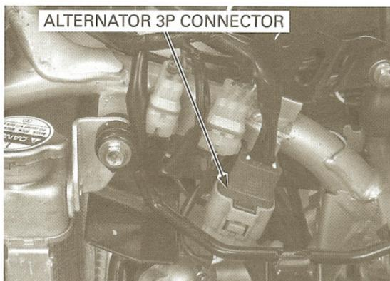
Measure the resistance between the Yellow wire terminals of the alternator side connector.
