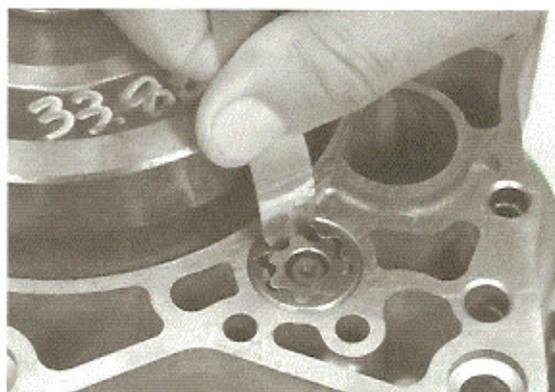
Measure the pump body clearance.
