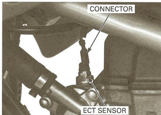
Suspend the ECT sensor in a pan of coolant (50 – 50 mixture) on an electric heating element and measure the resistance through the sensor as the coolant heats up.
