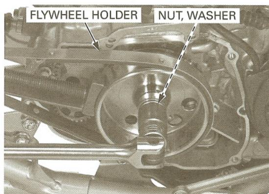
Remove the flywheel using the special tool.
