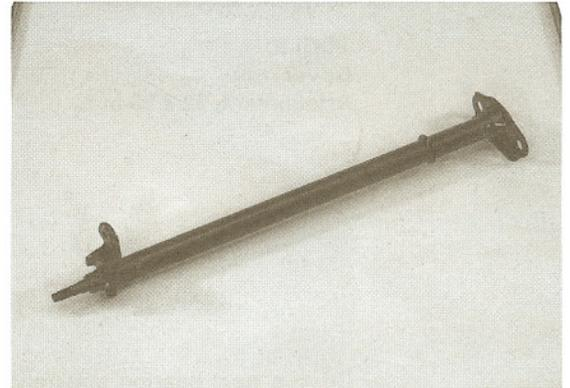
Turn the inner race of the steering shaft bearing with your finger. The bearing should turn smoothly and quietly. Also check that the bearing outer race fits tightly in the frame.
